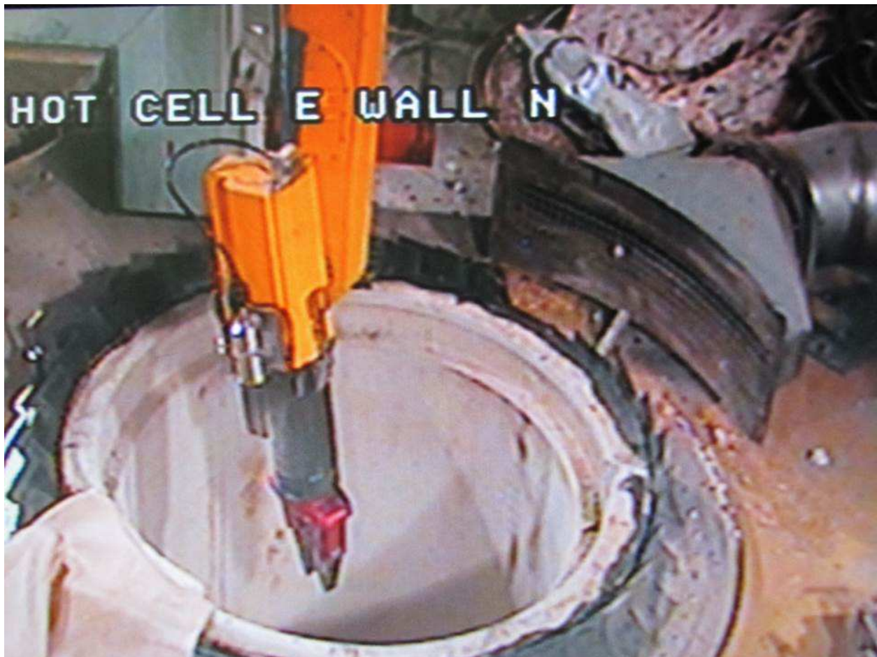
Fig. 1. Post Outage Manipulator Entering a Cask
