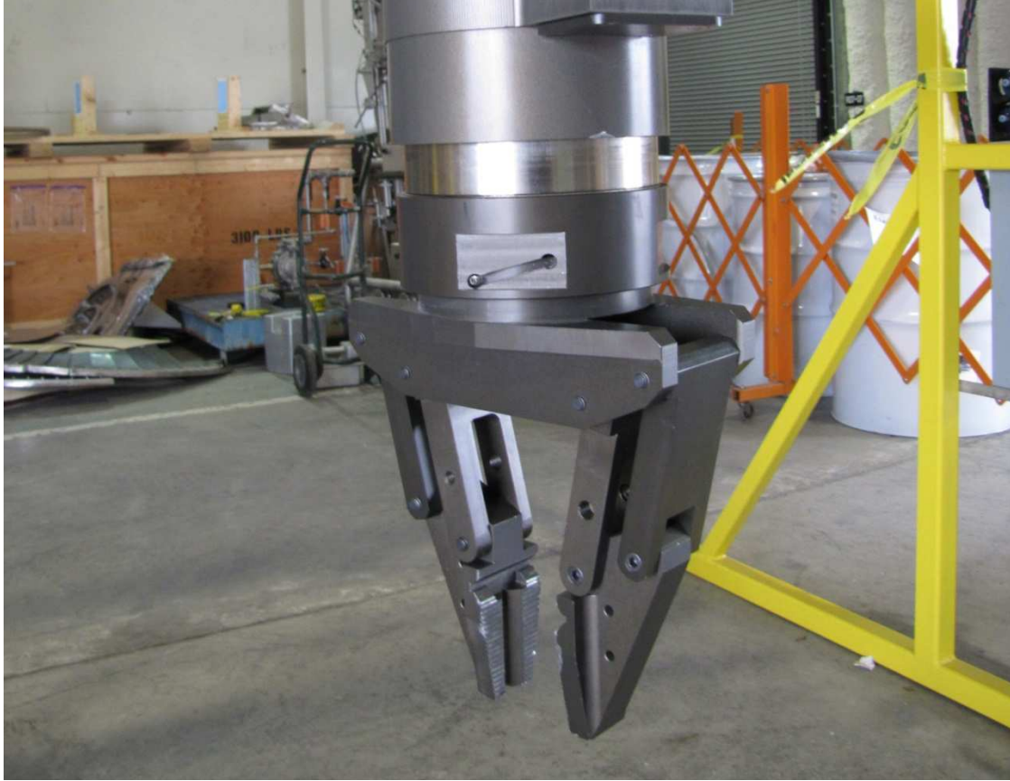
Fig. 7 Re-Designed Parallel Acting End Effector
