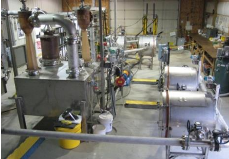
Fig. 4 GeoMelt system planned for install at NNL Central Lab, during construction acceptance testing.
