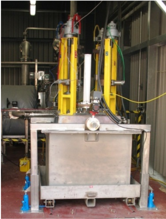
Fig. 5 GeoMelt 100 litre ICV treatment vessel, setup for UK waste trials in the UK.
