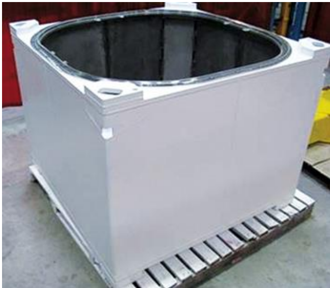
Fig. 6 Generic 3m3 container considered as future GeoMelt ICV container.
