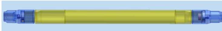
Fig. 9: Screwed particle-tight and gas-tight fuel rod capsule for transport of failed fuel rods and damaged fuel rods (with potential loss of nuclear material)
