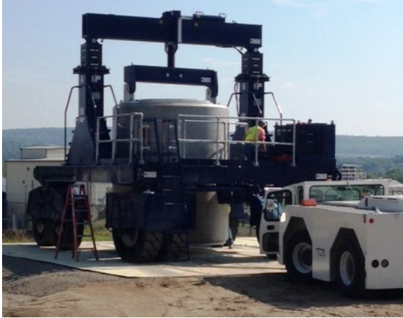
Fig. 6. Vertical Cask Transporter and GT50 Tugger positioning a cask
