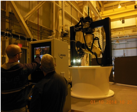
Fig. 10 and Fig. 11. Welder in use on mockup of VSC and overpack. Close-up of overpack weld.
