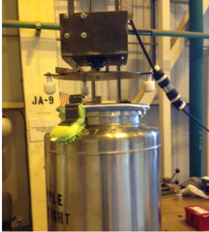
Fig. 16 and Fig. 17. Canister decontamination system mockup and decontamination pad carrier.
