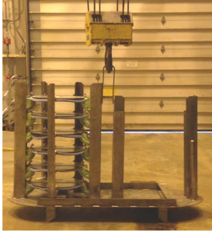
Fig. 16 and Fig. 17. Canister decontamination system mockup and decontamination pad carrier.
