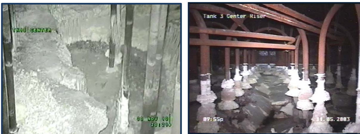
Figure 2. Dry Saltcake Prior to Dissolution in Tank 10 (left) and “Christmas Tree” Saltcake Formation on Tank 3 Cooling Coils Following Interstitial Liquid Draining (right)
