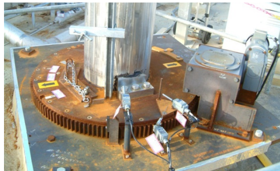
Figure 8. Mixing devices may be rotated continuously (oscillating), or may be focused on a particular area of the tank (indexed). Pictured is a Rotek system with installed SMP.
