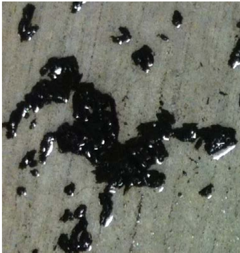
Fig. 5. Black gelatinous well foulant removed from injection well.
