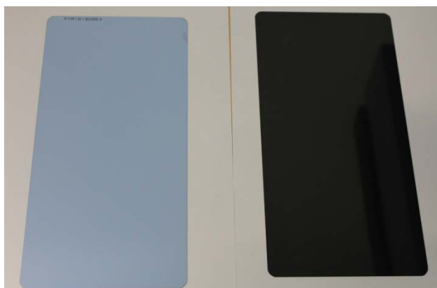
Fig.1. Phosphor screen used in the study; left: sensitive side, right: back side; type: TR, commercialized by Perkin Elmer; size: 12.5 x 25 \text{cm}^2
