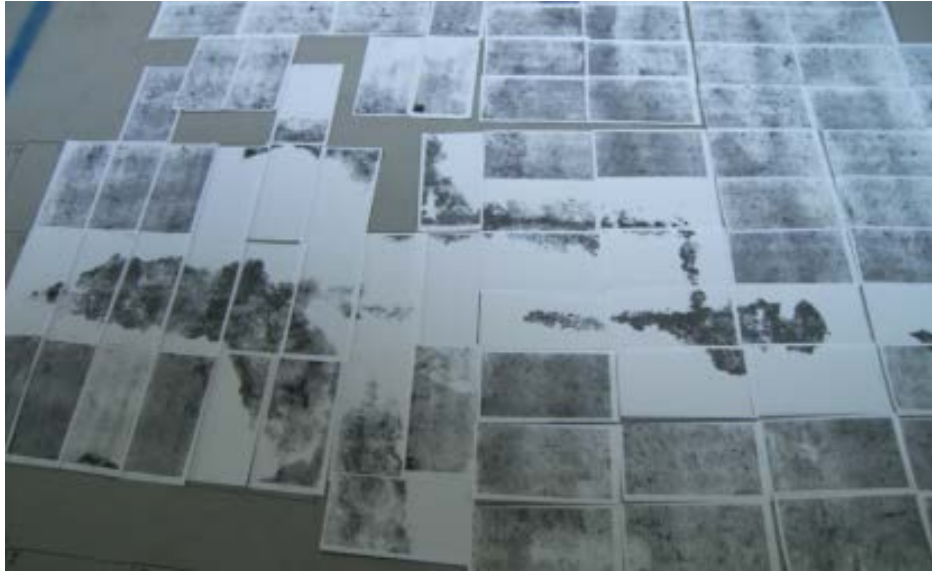
Fig. 4. Image of C-14 (50 000 Bq/g) on the floor of a facility
