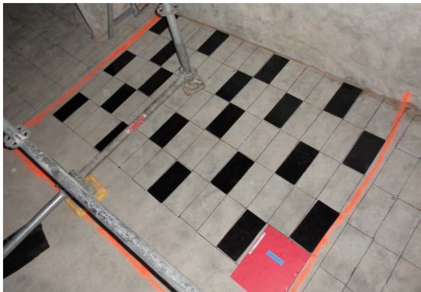
Fig.2. Batch of films (20) deposited on the floor of a facility
