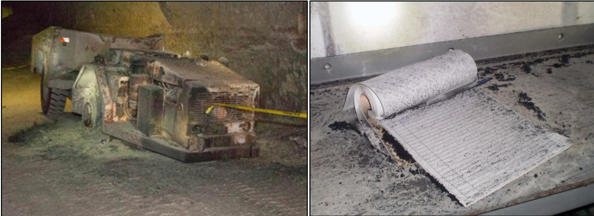
Fig. 2. Photos of Truck Fire and Soot Deposited on Surfaces in North Experimental Area of WIPP
