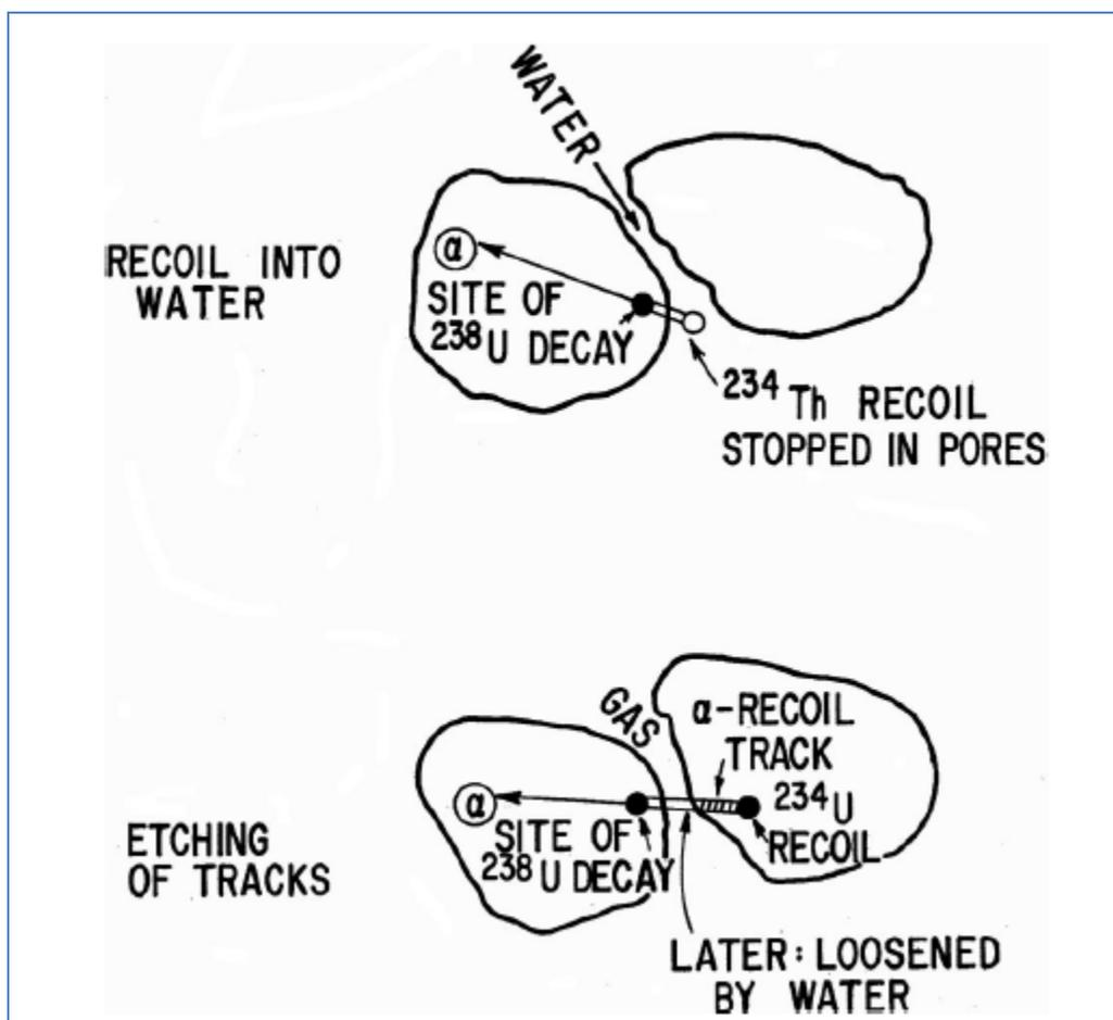
Figure 3 – Alpha Recoil Process
