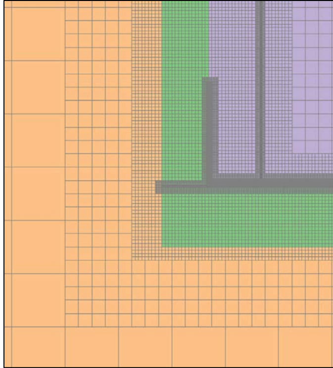
Fig. 8. Structured AMR grid implementation for submerged tank scenario showing four refinement levels at 4x each (profile view).
