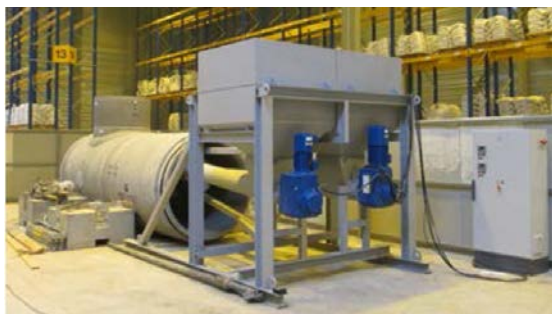
Fig. 8 - The metric test emplacement for bentonite admixture
