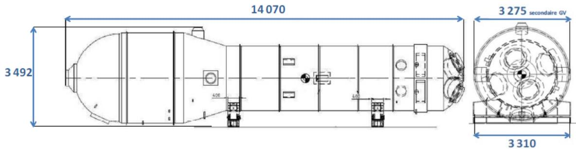
Fig. 2. Outer dimensions of the steam generators.
