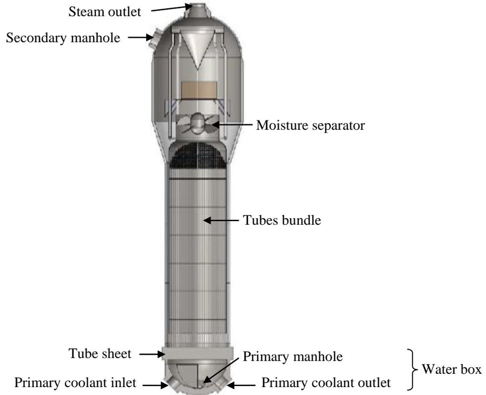
Fig. 1. Cross-section of a PWR steam generator.
