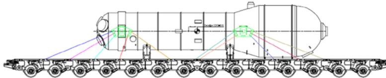
Fig. 10. Illustration of the 14-line trailer used.
