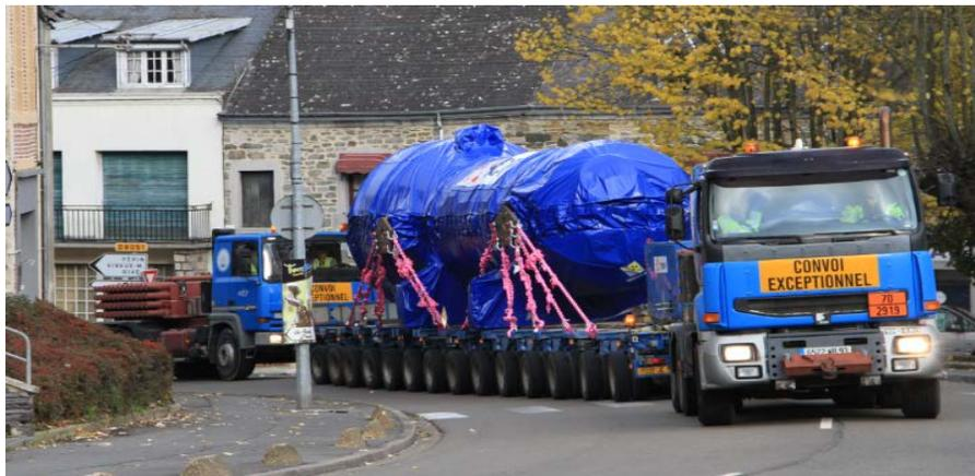
Fig. 11. One of the four SGs transported from Chooz A to the ANDRA VLLW repository, on a 14-line trailer with one pull truck and one push truck.
