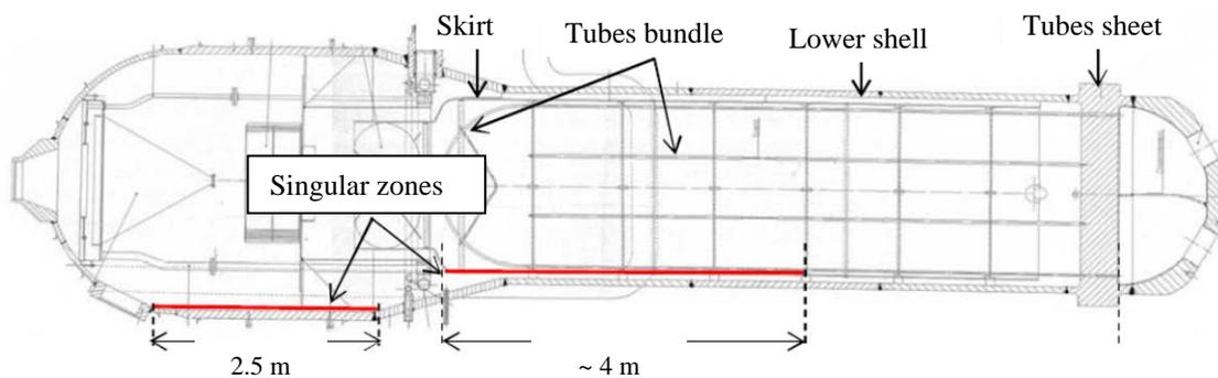
Fig. 7. Zones of the SG4 where residual activity was detected.
