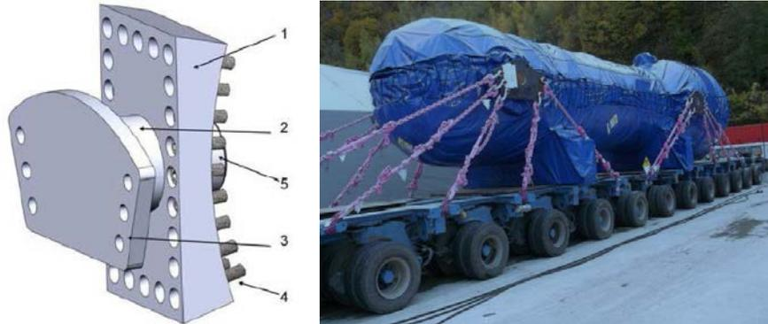
Fig. 9. System of plates used for the attachment of the chains.
