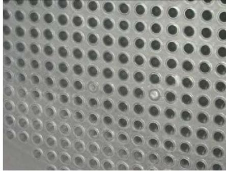
Fig. 3. Sealed tubes.
