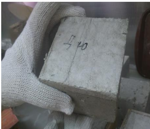
Fig. 1 Sample of diatomite cement 10x10x10 cm
