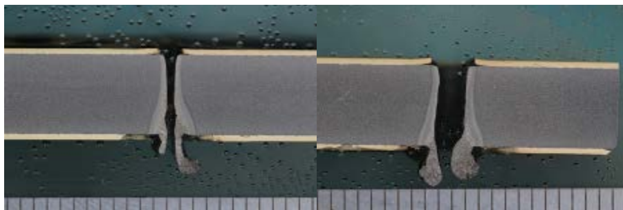
Figure 7 Cross-sections of laser cut kerfs produced in a 6mm thickness skip plate using 8bar cutting gas pressure with two SDs; 15mm (left), 50mm (right)
