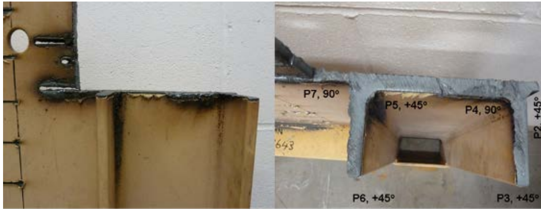
Figure 8 Laser cut edges and skip furniture cut section produced using optimised cutting sequence
