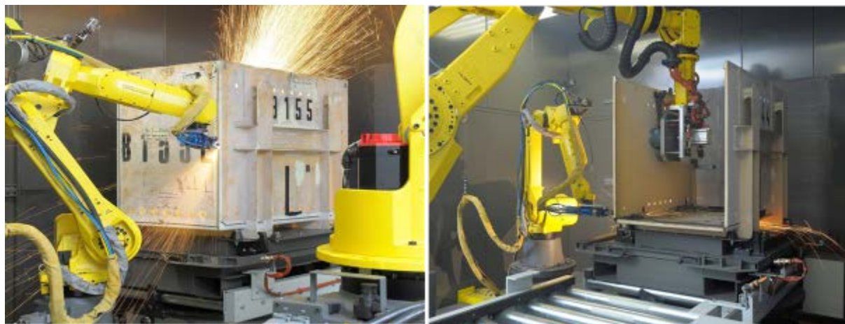
Figure 10 Laser cutting of an active skip at HPA: Laser cutting of face 1 (left); Laser cutting of stitches on face 2 (right).
