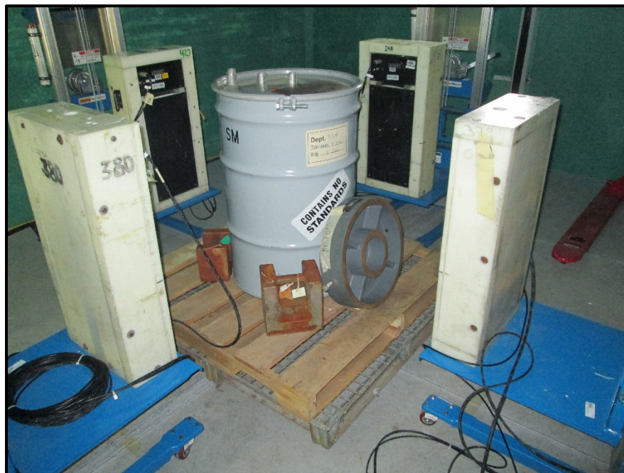
Fig. 4 Spallation Neutron Background Correction Measurement Configuration.
