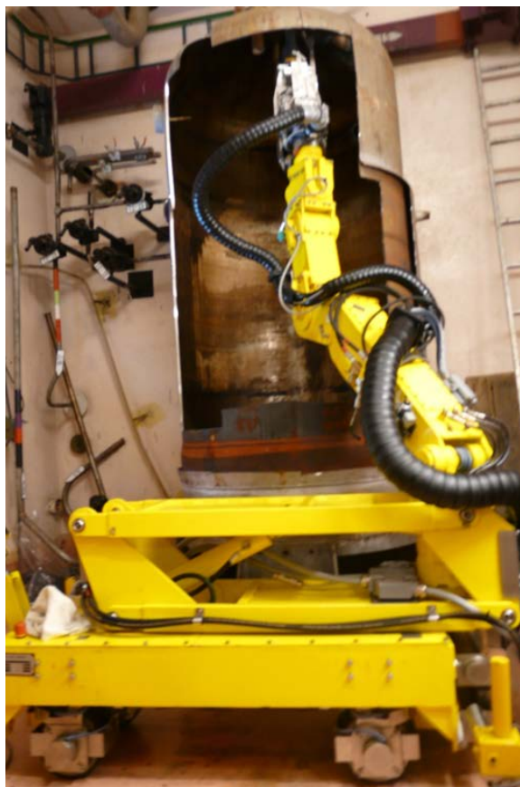
Figure 4. Manipulator MT 80 in operation
