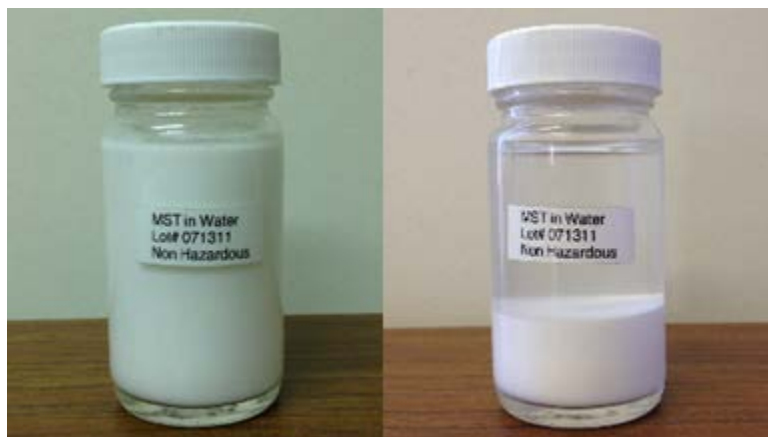
Figure 2: 15wt% MST Settling after Suspension (left) and after 24 Hours Settling (right)
