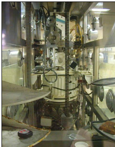
Figure 2 : Furnace inside the glove box
