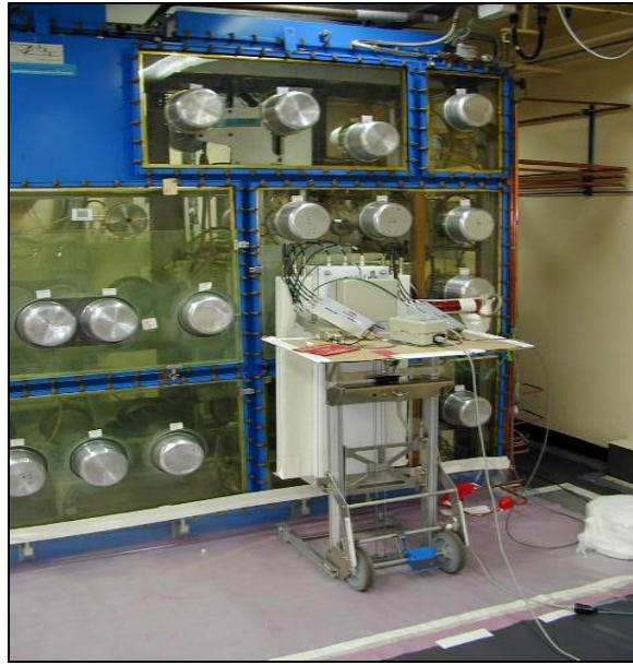
Figure 6 : Neutron slab in front of the glove box
