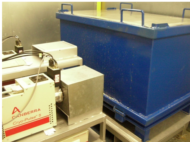
Fig. 2. Large Capacity Monitoring Post (LCMP)
