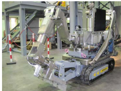
Figure 8: Cybernétix industrial version of a Brokk 90 equipped with an on-board controller and the Maestro arm. Tool rack on the front of the machine.
