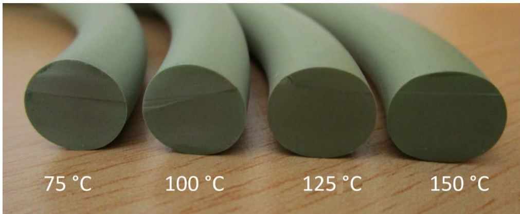
Fig. 12. Compression set of FKM after 100 d of aging at the indicated temperatures.
