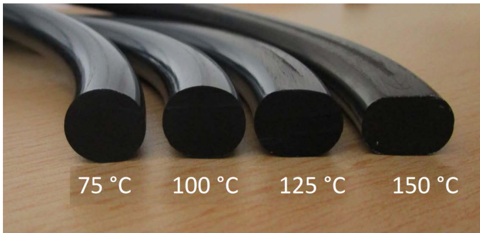
Fig. 11. Compression set of EPDM after 100 d of aging at the indicated temperatures.
