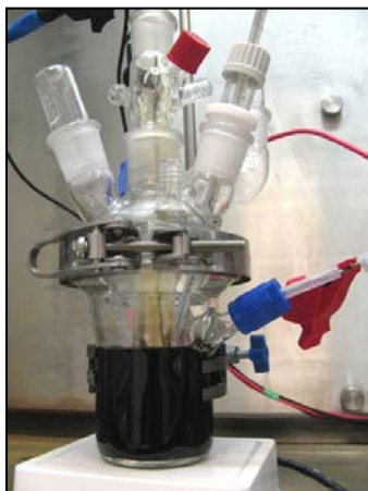
Figure 2. Experimental setup for 100 ml dissolutions using electrochemically generated Ag 2+
