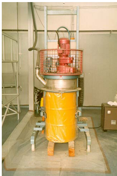
Fig 5. In-drum cementation unit.
