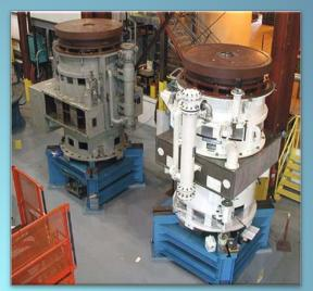
Alaron's fully equipped motor shop includes 2 large disassembly stands, a 15kV test panel and test stand, a Blu-Surf burnout/bakeout oven, and a 60 ton overhead crane with a 15 ton independent auxiliary hook.
