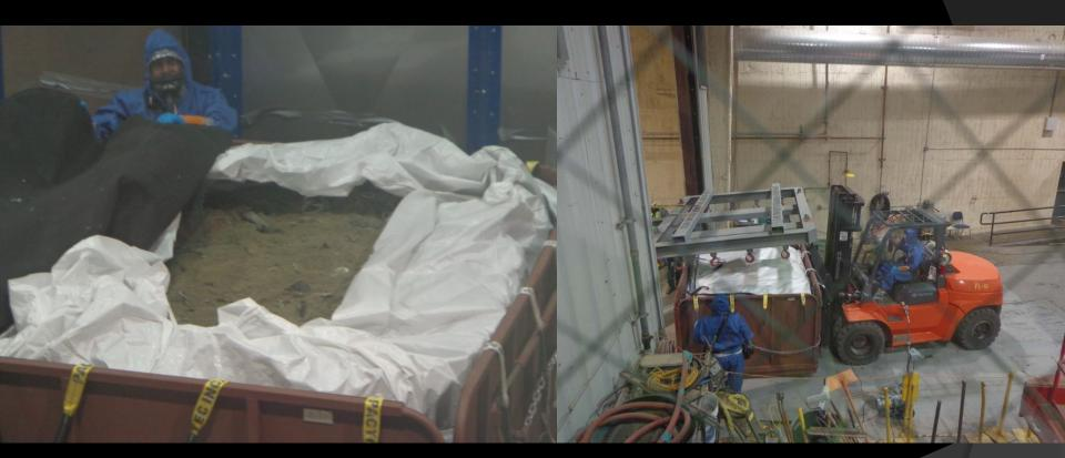
WCS workers perform stabilized treatment for shredded drum waste and then place the treated waste into flexible packaging for MLLW Class C disposal into FWF.
