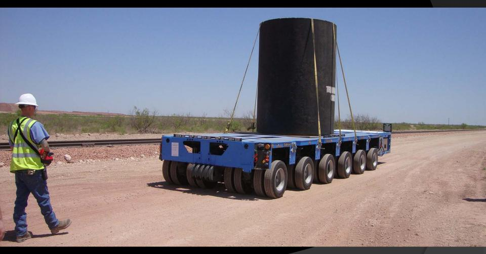
WCS has significant in-house capabilities to manage large component disposal. A worker is shown remotely driving a 60 ton MCC to a staging area.
