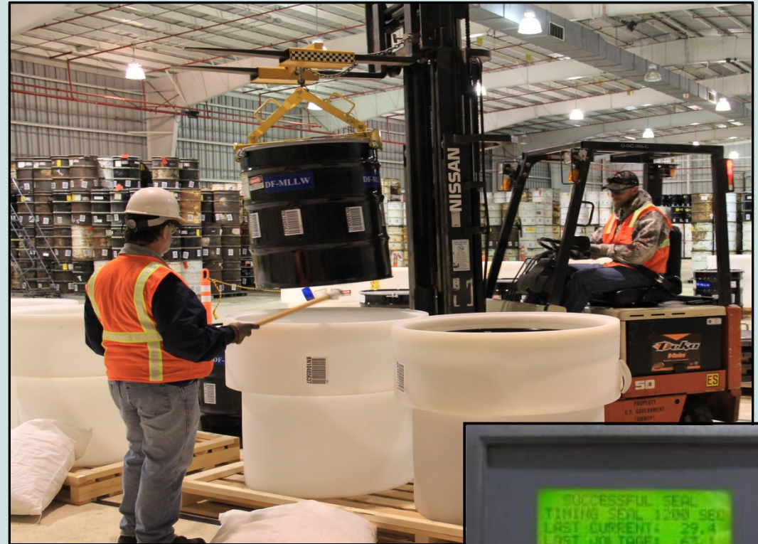
A product drum containing Mixed Low-Level Waste is lowered into a high density polyethylene "macro-pack." The lid of the macro-pack contains heating wires. An electric current is sent through the wires to permanently seal the container.
