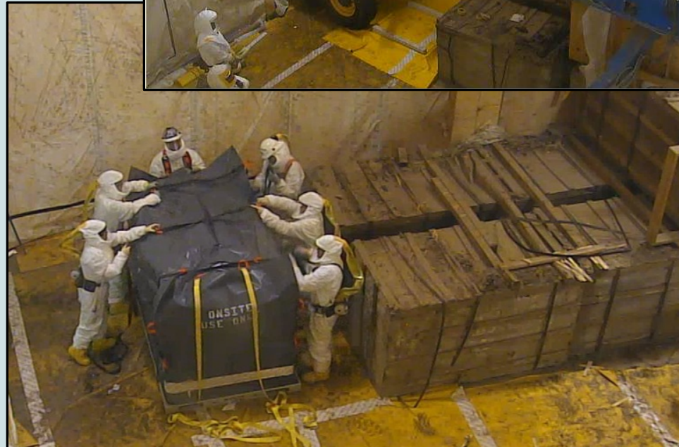
Employees retrieve a degraded wooden box using an employee-designed Box Retrieval Forklift Carriage (BRFC). Below, employees wrap degraded box with new soft-sided overpack used for deteriorating wooden boxes.
