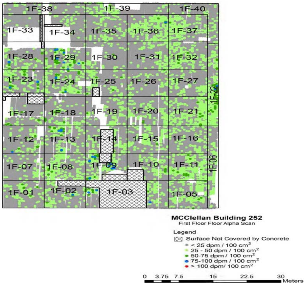
Figure 4.3-4 Building 252 1 st Level Floor Survey Units; Final Status Survey (Post Decontamination)
