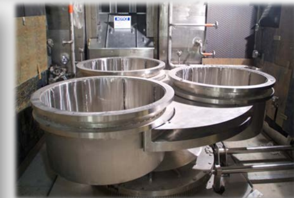
Canister drums are set on the melter turntables at the Low-Activity Waste Facility
