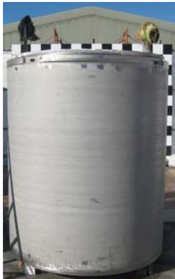
HIC with Reinforcement
