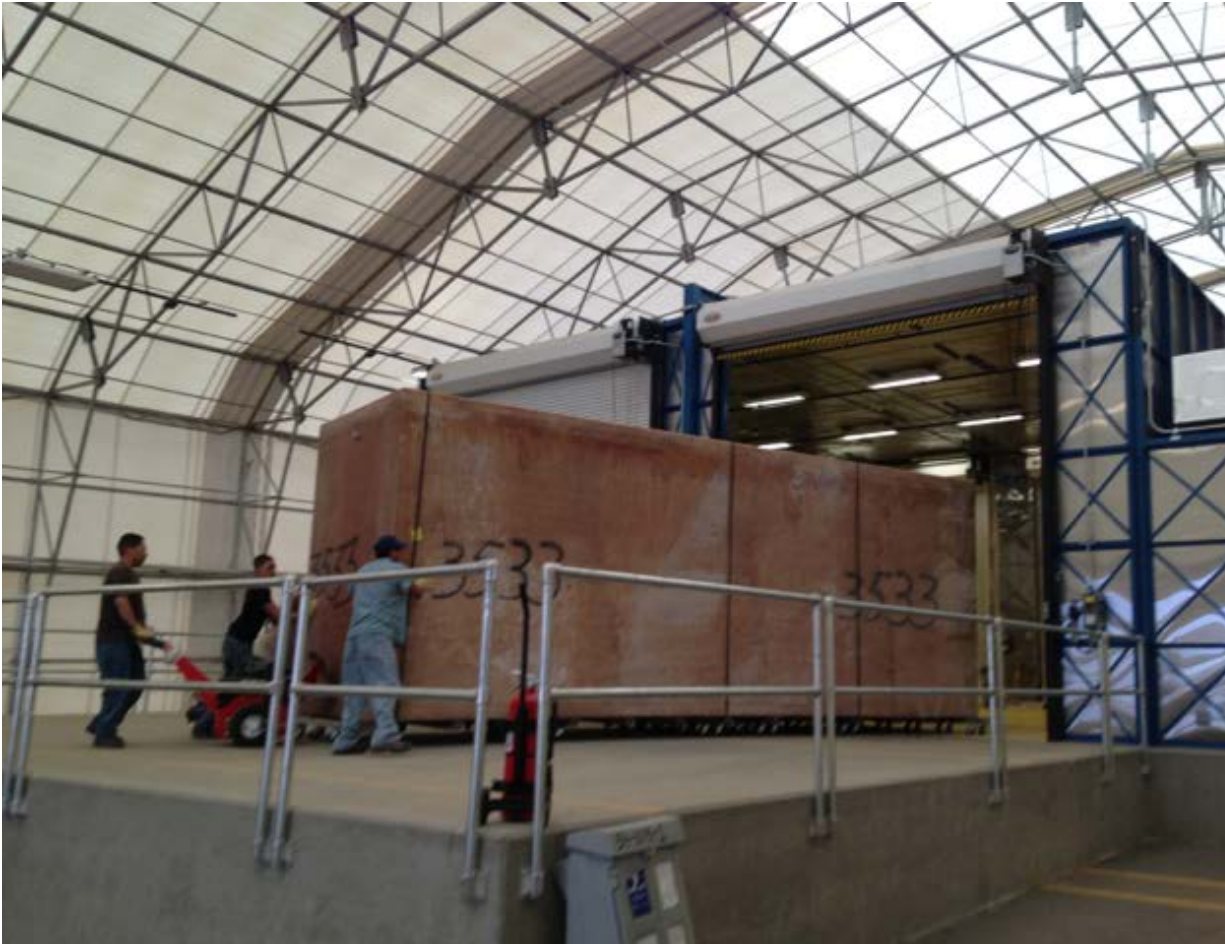
Photo 1 – Large TRU Waste box known as “The Bus”
