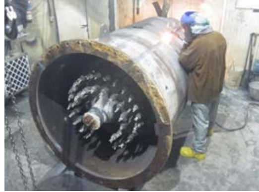
Fig.10. Cutting one of the pieces dismantled from the Pressurizer
