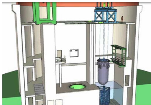
Fig. 12. Engineering plan for segmenting the reactor vessel.
