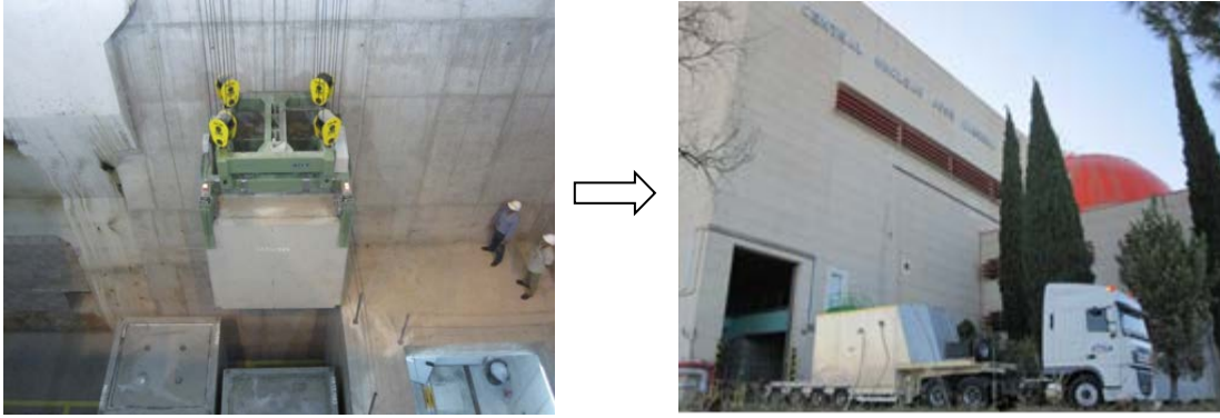
Fig. 5. The waste is packaged in concrete containers for shipment to El Cabril.
