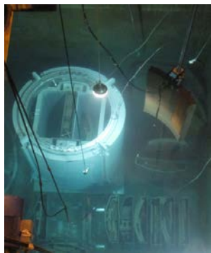
Fig. 6. Special waste load containing the reactor internals.
