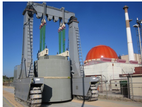
Fig. 7. Transport of HI-SAFE container to ITS.
