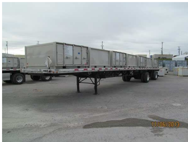
Figure 2. Reusable DOT 7A Type A Fissile Tested metal box.
