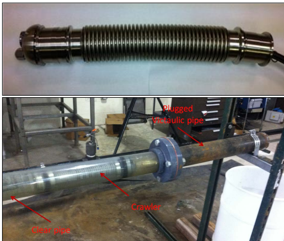
Fig. 1. Peristaltic pipe crawler technology (top) and peristaltic crawler performing an unplugging operation (bottom).
