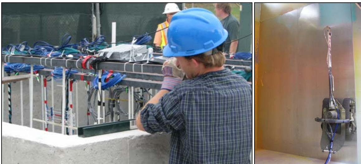
Fig 4. Installation of remote sensors at the ISD test site (left) and remote platform technology applying decontamination gel to vertical surface (right).
