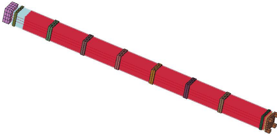
Fig. 2. Overall WE 17×17 OFA PWR fuel assembly sub-model (w/o control components, spacer blocks, or basket).
