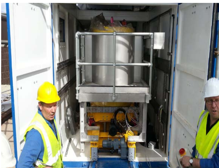
MOSAIK® container transfer bogie undergoing FAT tests inside and outside the container
