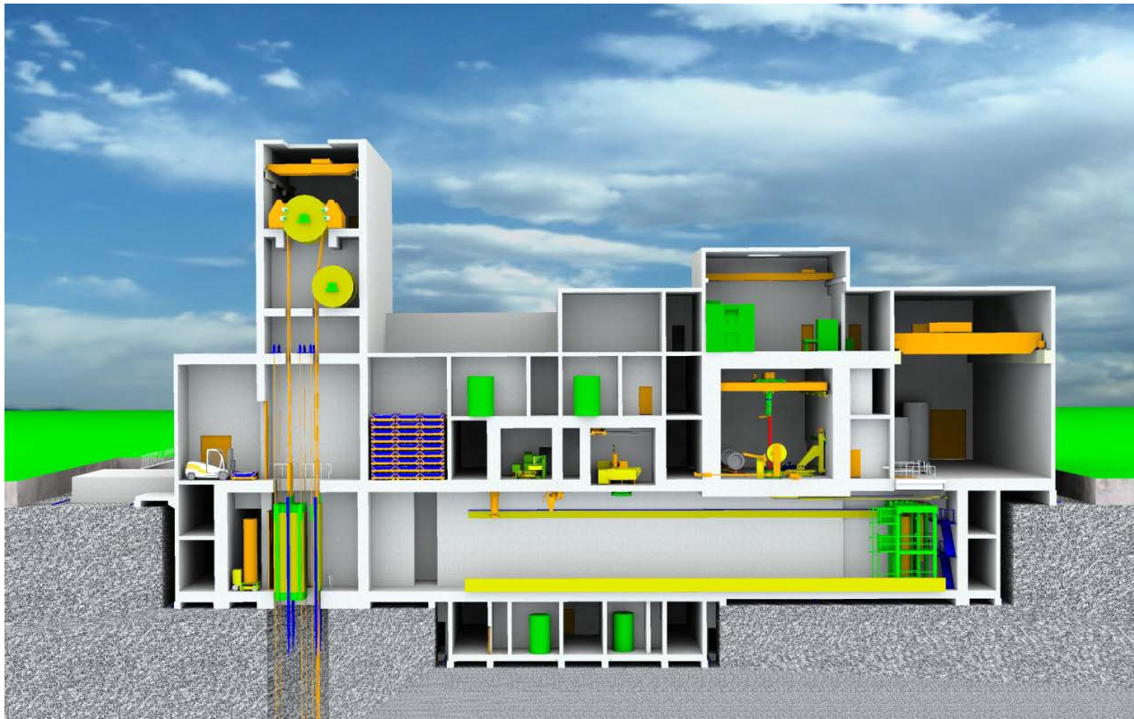
Fig. 7. Cross-section of the encapsulation plant. The receiving and storage areas for transport casks and new canisters are seen on the right. To the left of them are the fuel handling cell, the canister welding station, the weld inspection station and the interim storage for bentonite buffer blocks (Kukkola 2012). [2]
