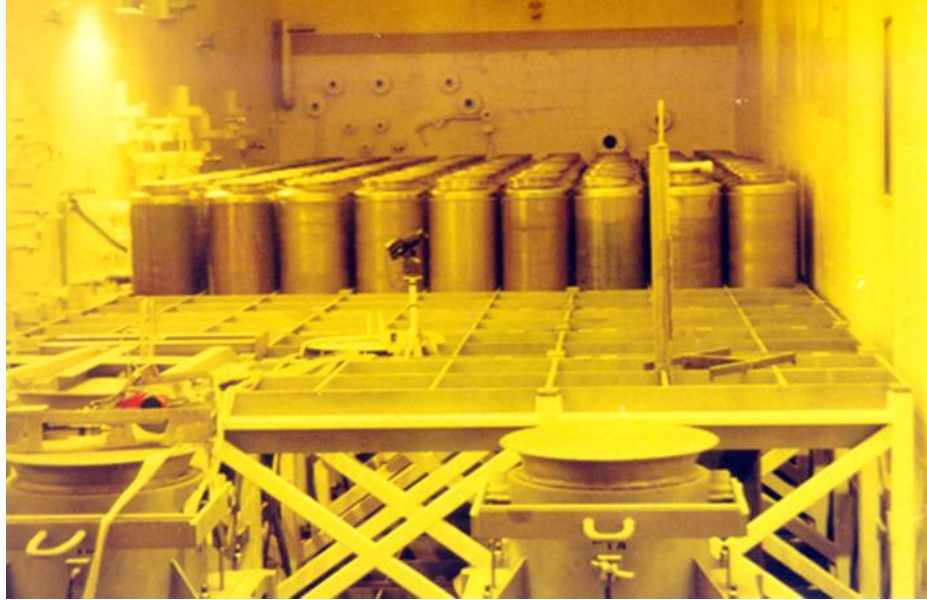
WVDP HLW Canisters in Racks in former CPC, looking South
