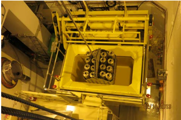
Fig. 9 Packing of loaded basket assemblies
