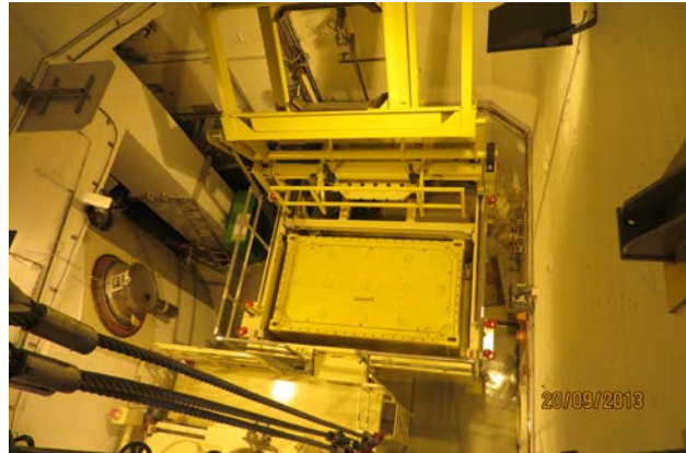
Fig. 10 Remotely controlled closing of the container
