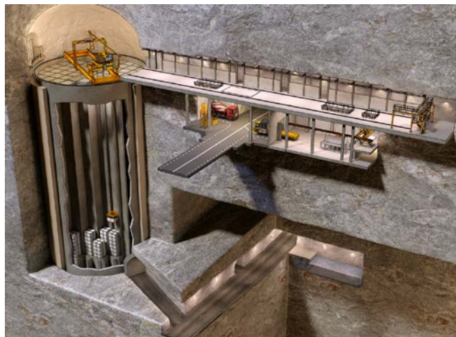
Fig. 2. Silo in SFR 1, for intermediate level waste with a surface dose rate of less than 500 mSv/h.
