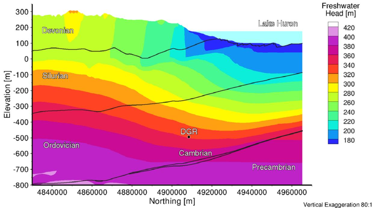
Figure 4: Reference Case Freshwater heads after 1,000,000 years simulation time.
