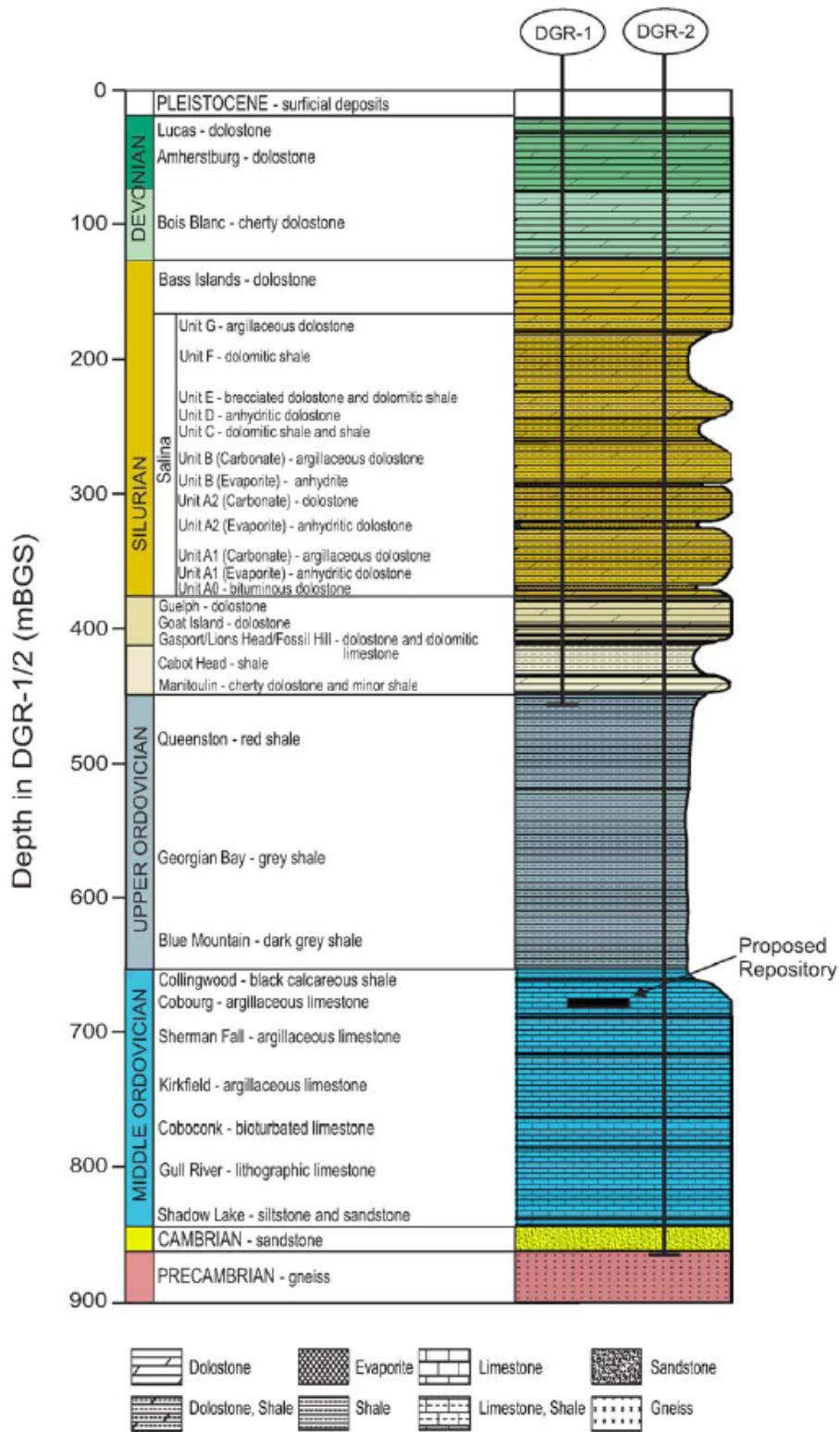
Figure 1: Reference Stratigraphic Column at the Bruce Nuclear Site Based Upon DGR-1 and DGR-2 Borehole Data. Figure from [1].
