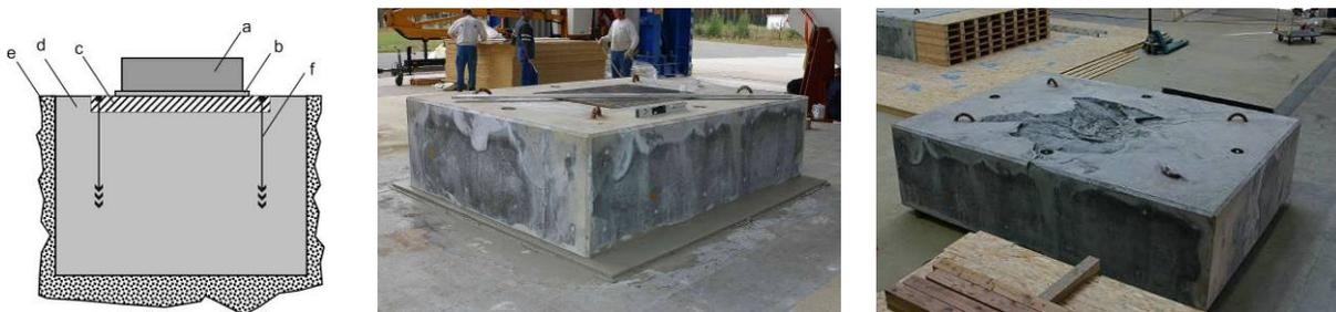
**Figure 5: Setup of the impact target for the drop tests with the KOBELCO waste container built of a reinforced concrete block adapted with mortar to the IAEA- target (left, middle) and the target locally destructed by the impact (right).**
