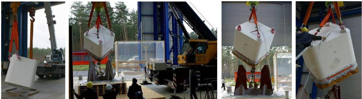
**Figure 6: Cask handling, positioning and adjustment of the container into the defined drop orientation.**
