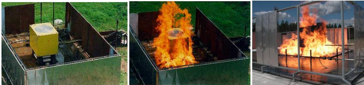
**Figure 11. Full scale one hour fire test with a cubic DCI container filled with ion exchanger resin (left and center; BAM Lehre); calorimeter test (right) with a cubic container (1.6 m x 2 m x 1.7 m) on the new open gas fire test facility (BAM TTS) with an achieved heat input of 75 kW/m<sup>2</sup> by low wind and a propane output rate of 2100 kg/h.**
