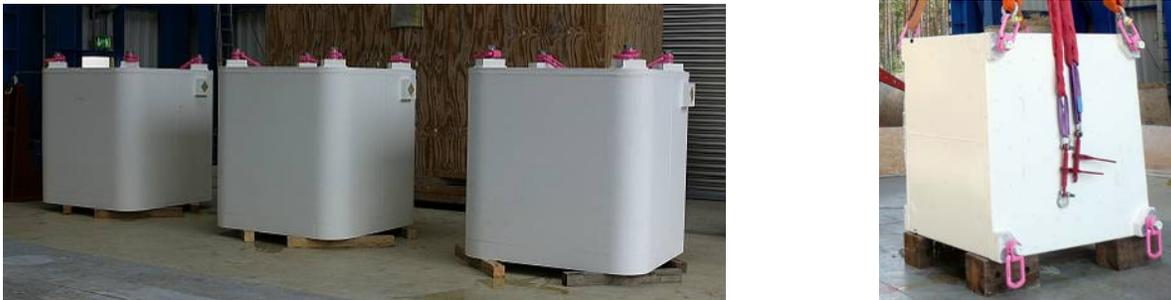
**Figure 2: Examples of drop tested international waste containers made of cast steel (left) and steel sheet (right).**
