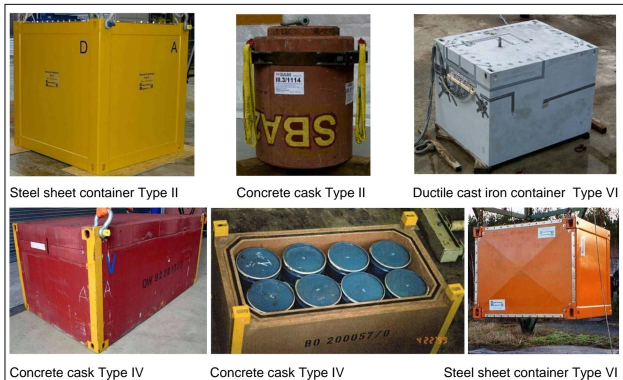
**Figure 1: Examples of drop tested national waste containers made from steel sheets, concrete or ductile cast iron**
