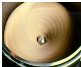
Fig. 2: Perfectly homogeneous concrete paste obtained with the Batch Mixer
