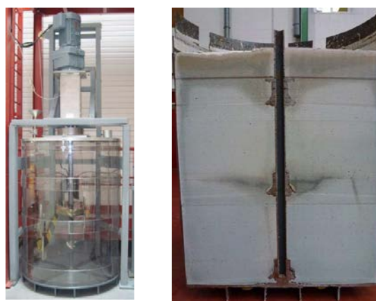
Fig. 3: In-drum test facility (left) and inside of a 1100 L drum after curing (right)
