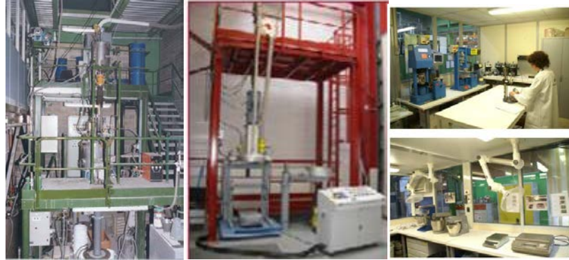
Fig. 5: AREVA's demonstration platform is used to test and qualify cementation and pre-treatment formulations in compliance with final waste package acceptance criteria
