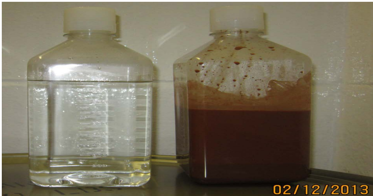
Picture 1 — After one million gallons processed. Left -Permeate Right Recirculated Solids Effluent
