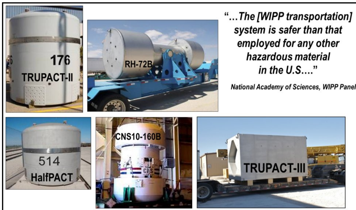
Fig. 3. WIPP Operates a Large Fleet of Different Waste Shipping Casks.
