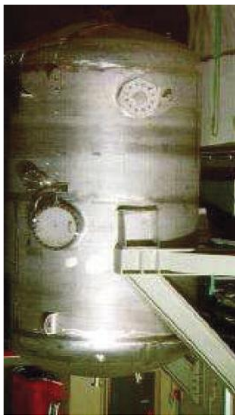
Fig. 4 - A water containing vessel of a type used in 'Wet Filtration' to solve the LOCA Vent Filtration problem
