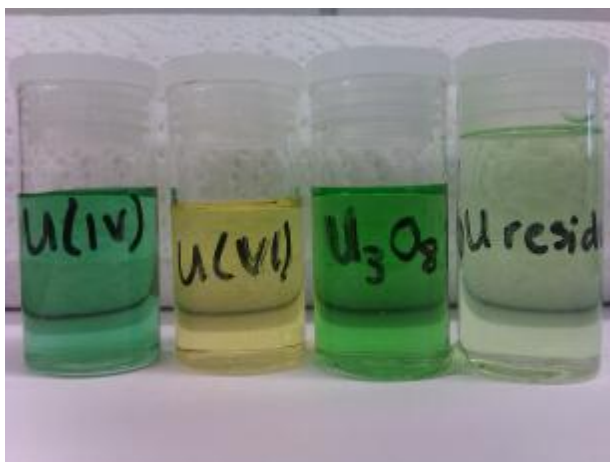
Fig. 4. U solutions in Na_2SO_4 -bearing H_3PO_4 Left-to-right: 0.0259 \text{ mol.dm}^{-3} U(IV) 0.0718 \text{ mol.dm}^{-3} U(VI) 0.0738 \text{ mol.dm}^{-3} U in U_3O_8 U residue solution
