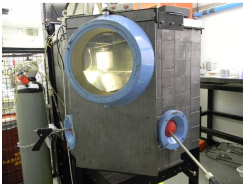
Fig. 8. Experimental hot cell for processing of irradiated U residue sample
