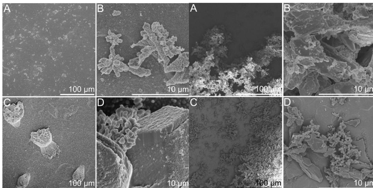
Fig 6. The surface of AISI/SAE 1005 detected with FE-SEM. A-B) Biotic environment, C-D) Abiotic environment.
