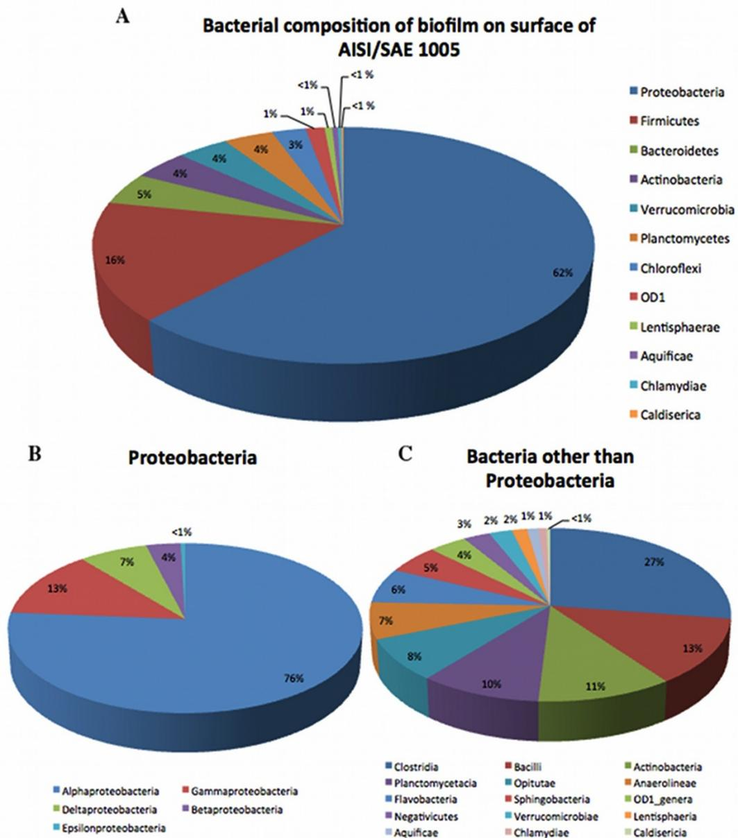
Fig. 3. A) The diversity and abundance of bacterial phyla detected on the surface of carbon steel AISI1005 after 12 months. All sequences of OTUs belonging to species within a phylum have been combined. B) The diversity and abundance of Proteobacteria. C) The diversity and abundance of bacteria other than Proteobacteria.
