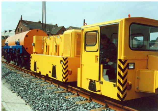
Fig. 5: DBE Transport System with Mining Locomotive and Transport Cart
